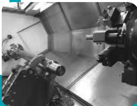
TOURNAGE CN 4 AXES CNC TURNING LATHES 4 AXES Ø 20 - 500 mm Length 10 - 3100 mm
